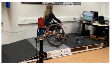
With the Lode Esseda wheelchair ergometer we can evaluate the wheelchair performance and propulsion technique of the wheelchair users in their own wheelchair. The most commonly used indicators of the wheelchair performance are the anaerobic and aerobic capacity. Both components can be measured on the wheelchair ergometer in a standardized, but individualized way. By doing so,
